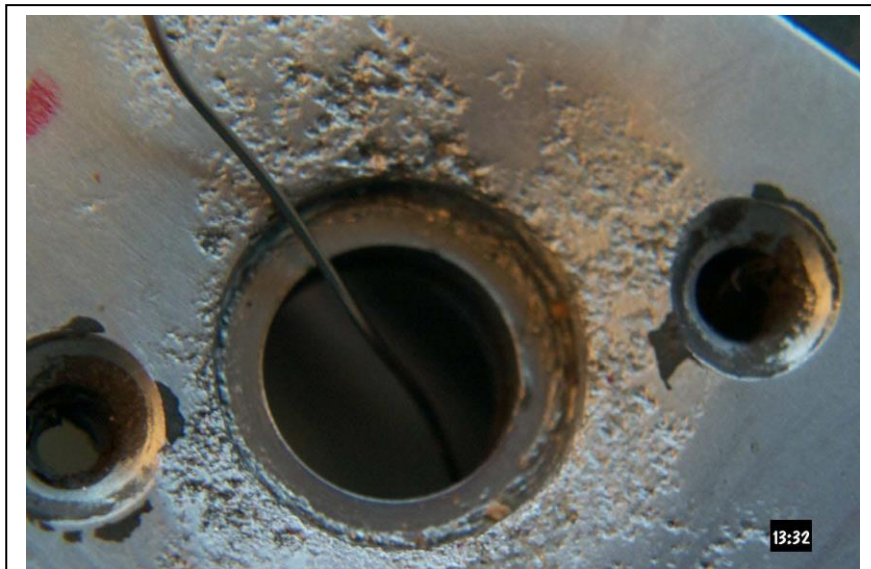
Figure 1. Airframe galvanic corrosion around F-18 wing-attach bushing.
