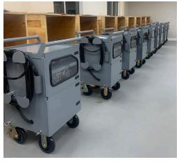
*Corrdesa LLC, GA USA, partnered with Dalic, France to produce the ruggedized, mobile Dalistick® system for ZnNi plating repairs directly on aircraft. Image Courtesy Corrdesa LLC, Distribution A: Approved for public release; distribution is unlimited.*
