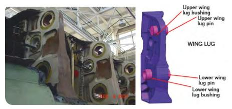
FIGURE 1 Corrosion in F-18 wing-fuselage attach bulkheads.8
