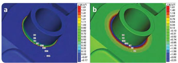
FIGURE 2 Corrosion currents for the wing lug assembly: (a) anodized AI, Cd-plated CuBe, and steel; (b) anodized AI, bare CuBe, and steel.
