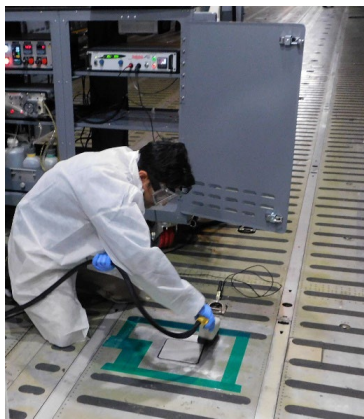
Figure 3. Re-anodizing C-5 cargo floor.
